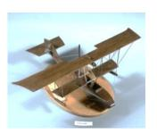
In **1912**, the French pilot and engineer François Denhaut built the **Donnet-Lévêque**, **the first flying boat**. For the first trials, Denhaut left the hull flat-bottomed. This caused a suction effect, so the craft was unable to take off. He then added an indentation under the hull, called a "step," which created an air bubble that overcame the suction and allowed the seaplane to lift off.
